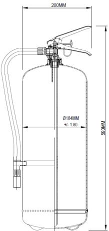
The 9KG powder extinguisher is suitable for construction sites, heavy industries, large vehicles, and areas requiring a higher coverage against incipient fires.
