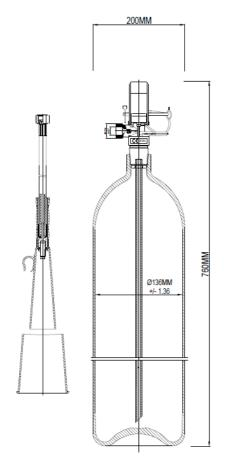
The is 5KG Carbon dioxide extinguisher is suitable for construction sites, heavy industries, large vehicles, and areas requiring a higher coverage against incipient fires.
