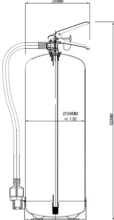
The 9L Water fire extinguisher is suitable for construction sites, heavy industries, large vehicles, and areas requiring a higher coverage against incipient fires.
