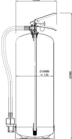
The 9LTR foam fire extinguisher is suitable for construction sites, heavy industries, large vehicles, and areas requiring a higher coverage against incipient fires.
